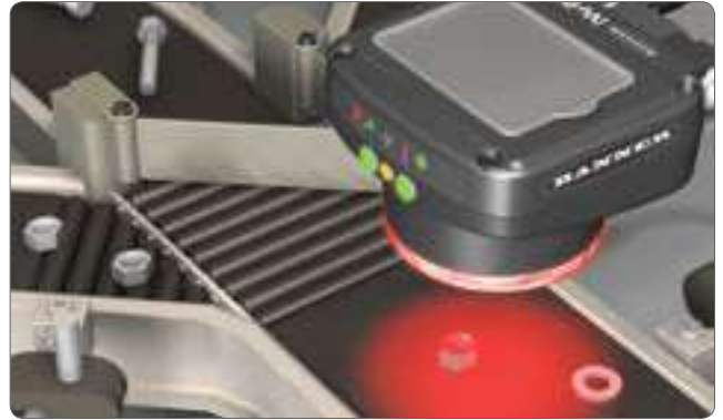
Hardware sortation using a Sort Sensor
