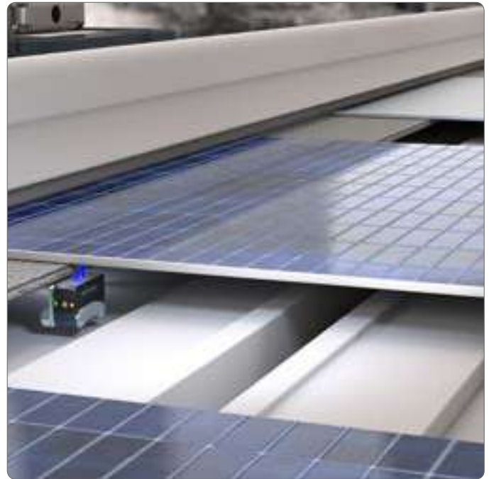
Wafer detection using the VS8
