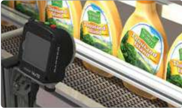
Label detection using a Match Sensor
