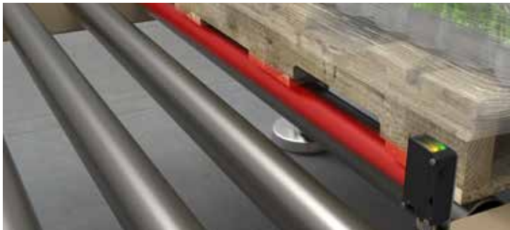
Wide-Beam Leading Edge Detection
