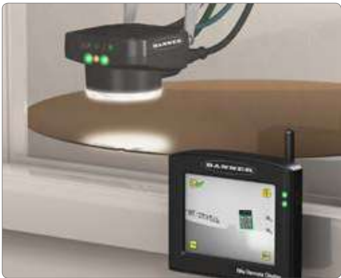
Barcode detection on semiconductor wafer
