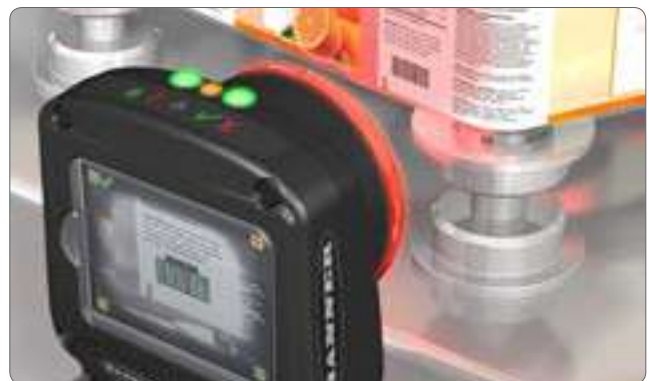
Label verification on labeler machine
