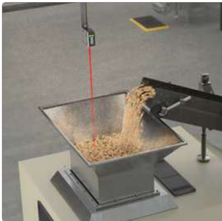
Monitoring levels inside a high-volume hopper
