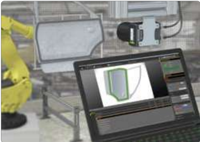
Door panel adhesive inspection using Bead Tool
