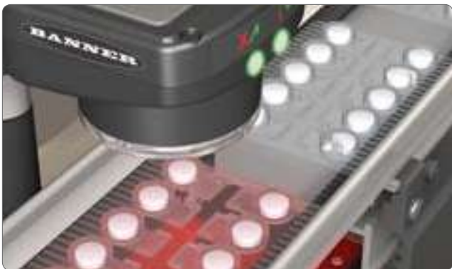
Blister pack inspection using an Area Sensor
