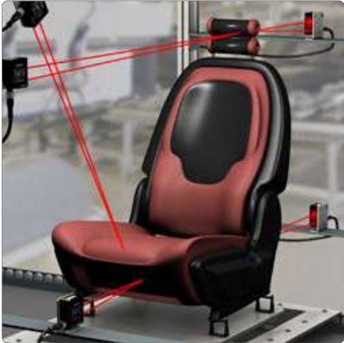
Auto seat adjustment measurement using the LE550
