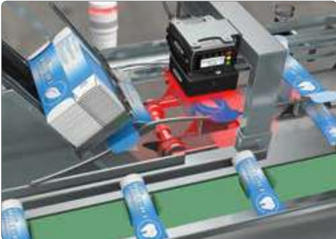
Correct carton inspection using Match Tool
