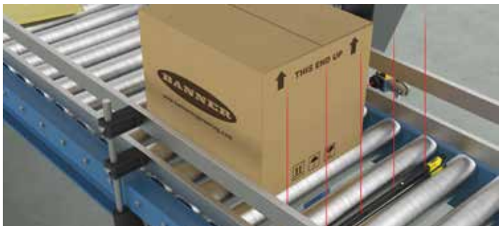
Through the Roller Leading Edge Detection
