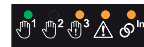
LED 1: Object Detection in Safety Zone (OSSD) LED 2: Not Available LED 3: Assigned to Warning Zone 2 LED 4: Assigned to Warning Zone 1 LED 5: Interlock Status (waiting for Reset)
