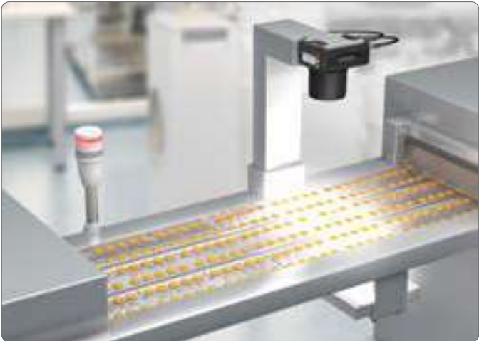
Blister pack inspection using BLOB Tool
