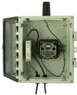
10 × 8 in: Fits a power supply, surge suppressor, a single DX80, and a few relays. This is a popular size but can get cramped.
