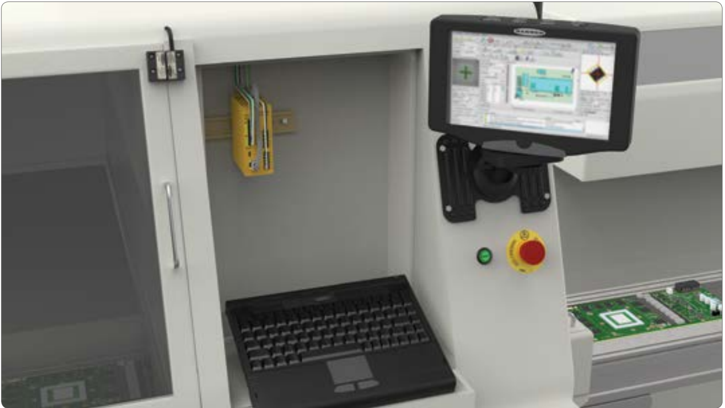
PCB Automated Assembly Station
